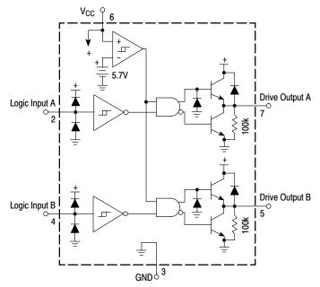
Figure 1. Representative Block Diagram
