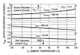
Figure 11. Drive Output Saturation Voltage versus Temperature
