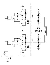
Output Schottky diodes are recommended when driving inductive loads at high frequencies. The diodes reduce the driver's power dissipation by preventing the output pins from being driven above  $V_{CC}$  and below ground.
