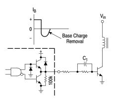
The totem–pole outputs can furnish negative base current for enhanced transistor turn–off, with the addition of capacitor  $C_1. \label{eq:constraint}$
