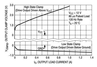
Figure 9. Drive Output Clamp Voltage versus Clamp Current
