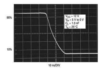
Figure 13. Drive Output Fall Time
