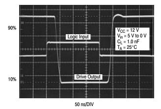
Figure 8. Propagation Delay
