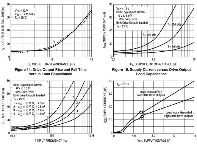
Figure 16. Supply Current versus Input Frequency
