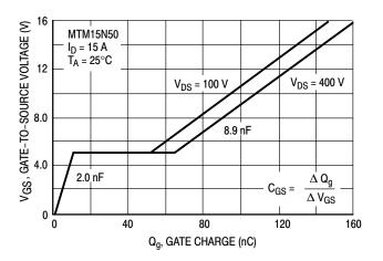
Figure 18. Gate–To–Source Voltage versus Gate Charge
