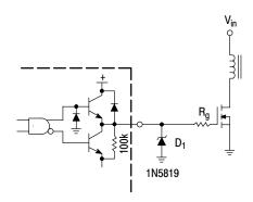
Series gate resistor  $R_g$  may be needed to damp high frequency parasitic oscillations caused by the MOSFET input capacitance and any series wiring inductance in the gate-source circuit.  $R_g$  will decrease the MOSFET switching speed. Schottky diode  $D_1$  can reduce the driver's power dissipation due to excessive ringing, by preventing the output pin from being driven below ground.
