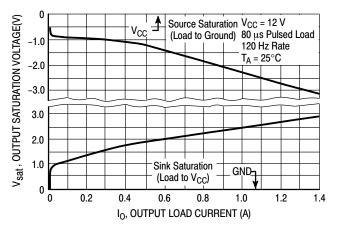
Figure 10. Drive Output Saturation Voltage versus Load Current
