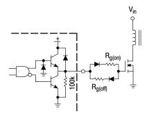
In noise sensitive applications, both conducted and radiated EMI can be reduced significantly by controlling the MOSFET's turn-on and turn-off times.
